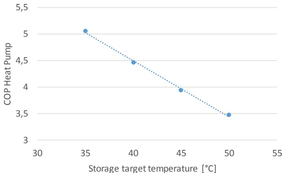
Fig. 7. Heat pump COP dependent on buffer storage temperature
