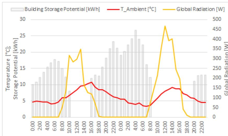
Fig. 8. Thermal storage potential of building mass
