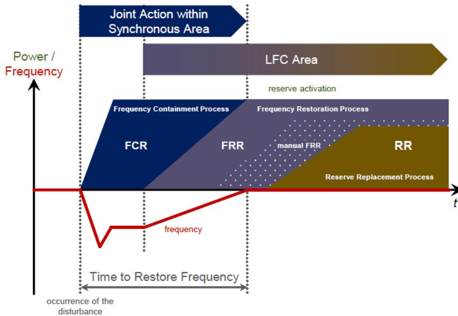
Fig. 4. Dynamic hierarchy of load-frequency control processes
