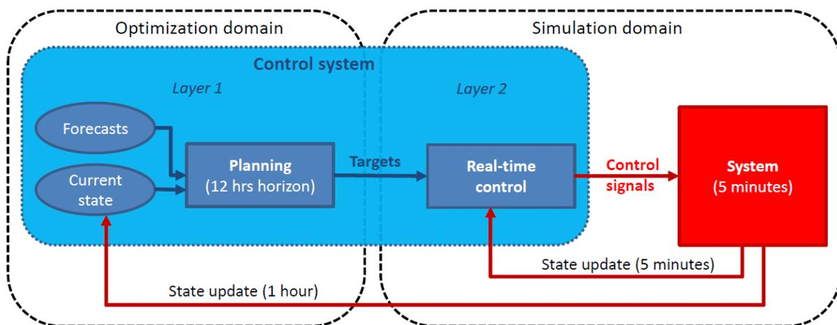
Fig. 15. Schematic overview of the advanced control logic. (Vivian, Jobard, Ben Hassine, Pietrushka, & Hurink, 2017)
