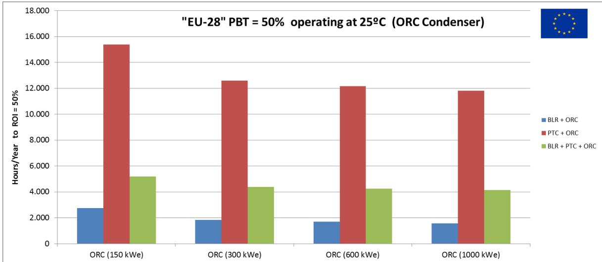
Figure 89 – PBT for EU28 in function of ORC scaling
