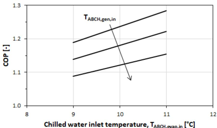
Figure 49 - Thermal COP of the absorption chiller as a function of the chiller water inlet temperature for different generator inlet temperatures (165, 170, 175  $^{\circ}\text{C}$ , increasing along the arrow direction) at  $28^{\circ}\text{C}$  inlet condenser temperature.
