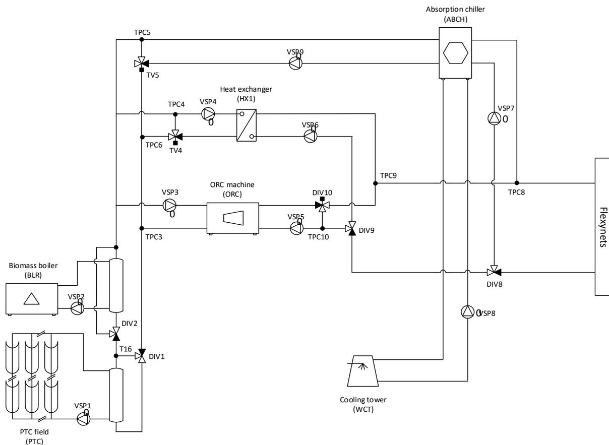
Figure 45 – Layout of power station.
