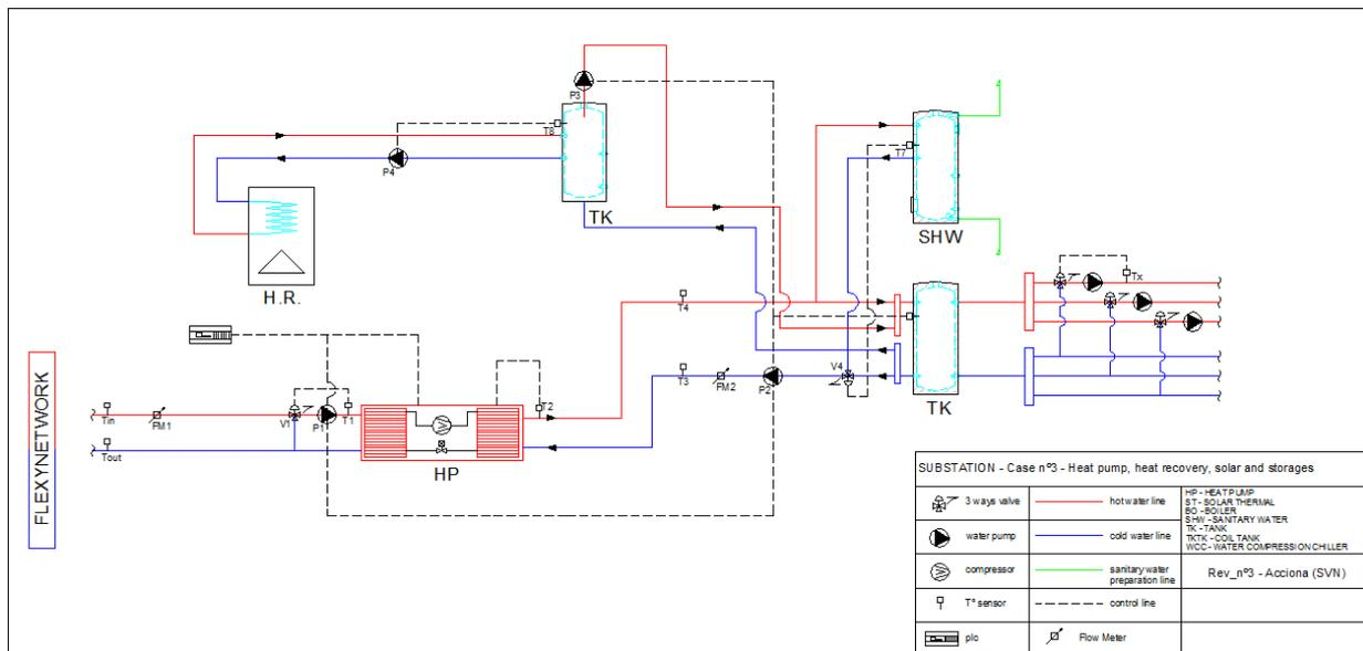
Figure 108 – Simplified lay-out for software implementation (4 pipes HP with HR)
