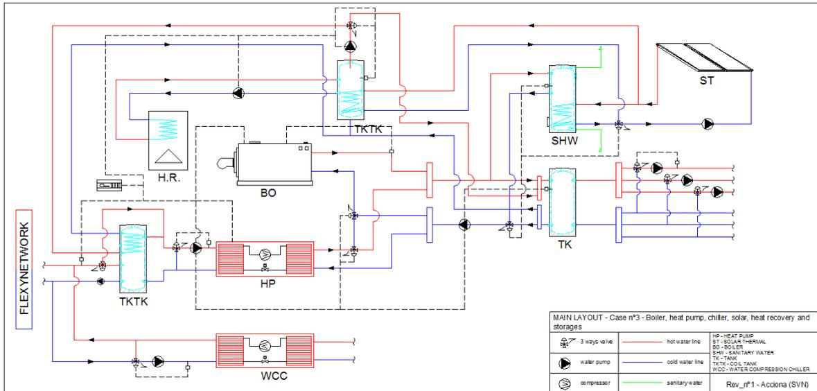
Figure 107 – Global P&ID for 4 pipes domestic sub-station with heat recovery
