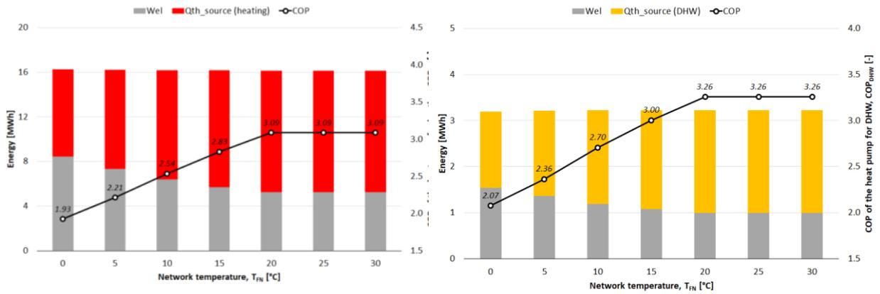
Figure 32 – Yearly energy balance for residential substations: existing (“EX”) SFH buildings for the location of Rome.
