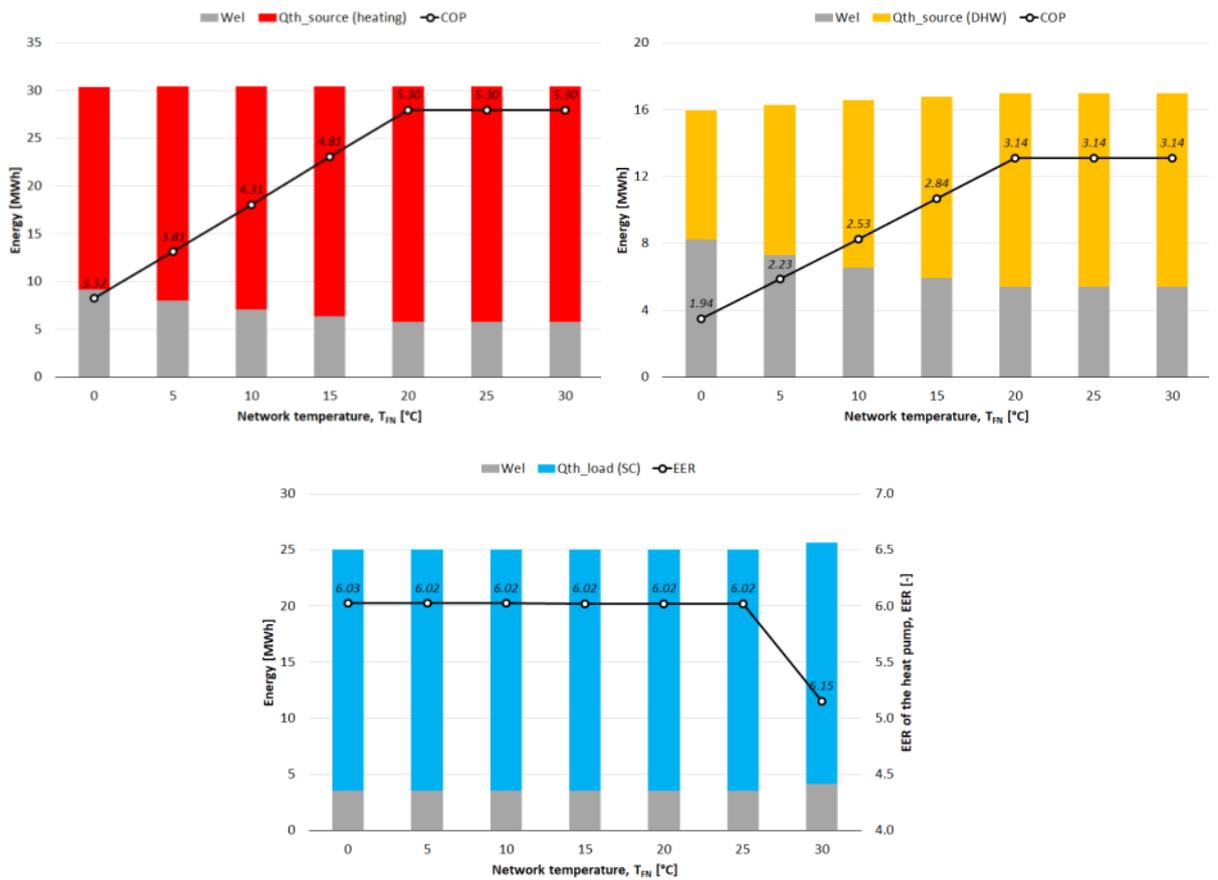
Figure 39 - Yearly energy balance for residential substations: new/renovated (“45”) s-MFH buildings for the location of Rome.
