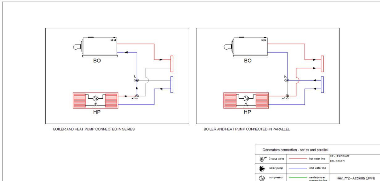
Figure 102 – Detail of connection boiler with HP
