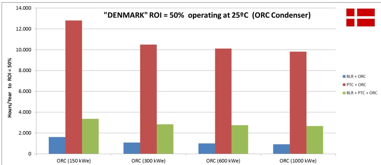
Figure 90 – PBT for Denmark in function of ORC scaling
