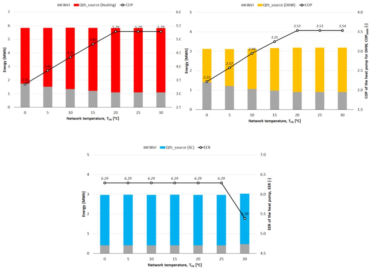
Figure 33 - Yearly energy balance for residential substations: new/renovated (“45”) SFH buildings for the location of Rome.
