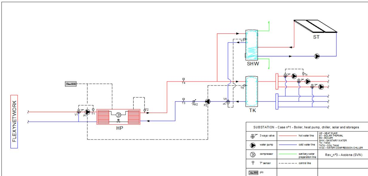
Figure 104 – Simplified lay-out for software implementation (2 pipes HP)
