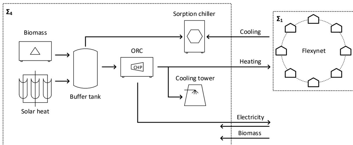
Figure 44 – Single line diagram of the energy system.
