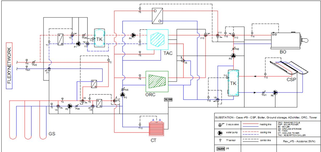
Figure 109 – Global P&ID for thermal powerstation
