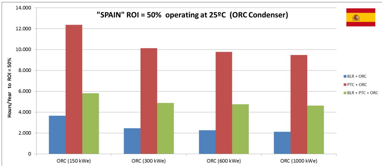
Figure 91 – PBT for SPAIN in function of ORC scaling
