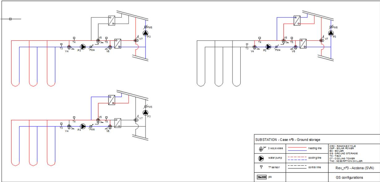
Figure 111 – Details of operation of the ground storage and network connection
