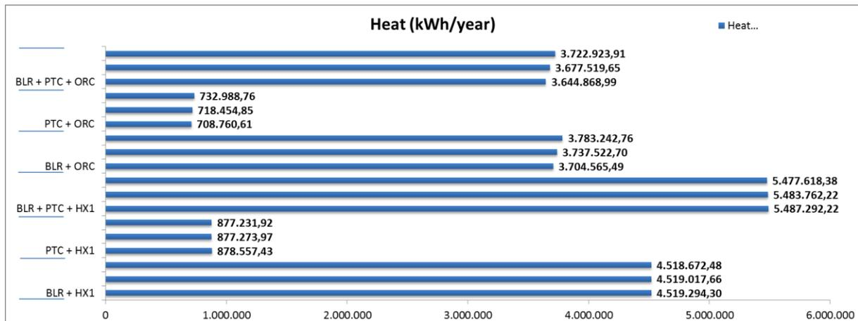
Figure 56 – Comparison of heating production between different Powerstation heating combinations.
