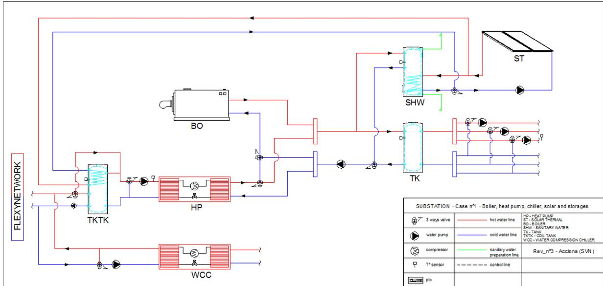
Figure 101 – Global P&ID for 2 pipes domestic sub-station
