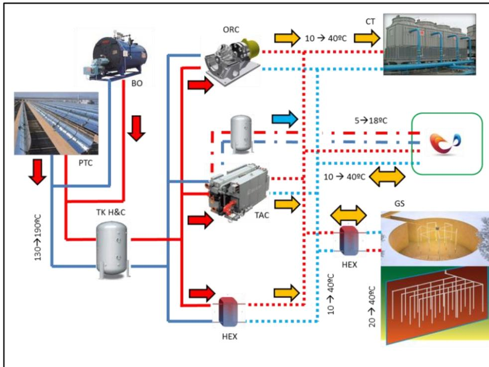
Figure 17 – PTC power station with FLEXYNETS.
