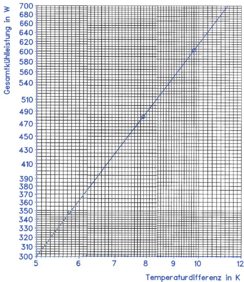
Figure 84 – Characteristic curve of the radiant ceiling TRIPAN®.
