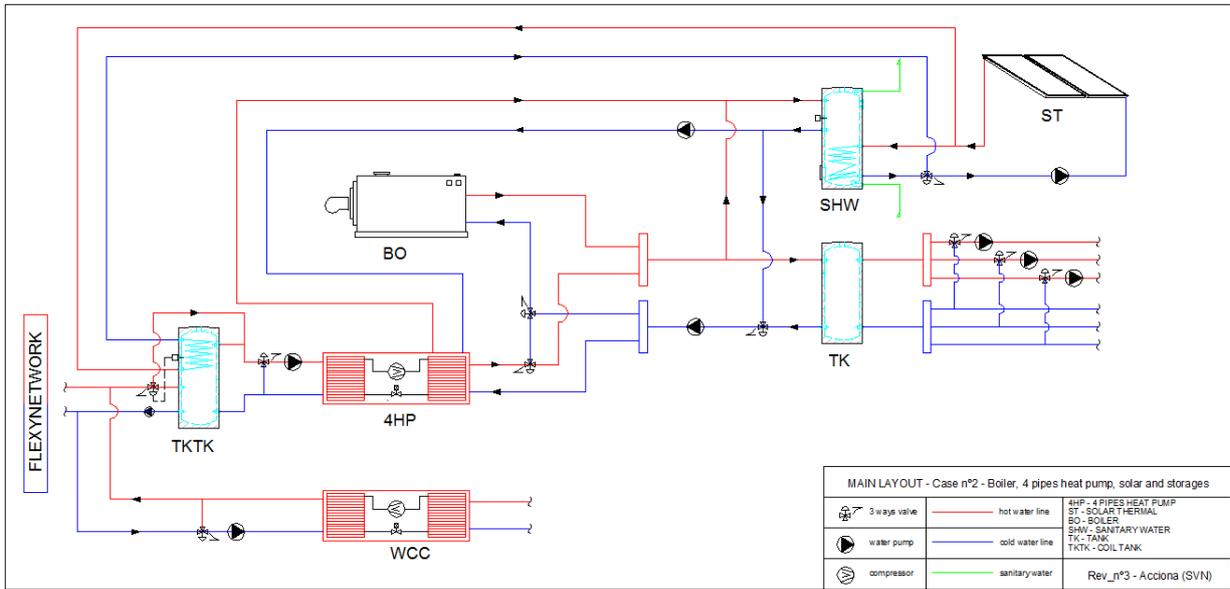
Figure 105 – Global P&ID for 4 pipes domestic sub-station
